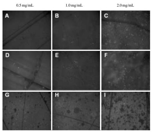
**Figure 3.** Fluorescence image of the diynePC layer on a glass surface. Various concentrations of diynePC were used for the vesicle fusion, 0.5 mg/mL (A, D, and G), 1 mg/mL (B, E, and H), and 2 mg/mL (C, F, and I). Vesicle fusion was carried out at room temperature for 1 min (A, B, and C), at room temperature for 30 min (D, E, and F), and above the transition temperature for 1 min (G, H, and I).
