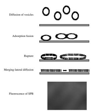
**Figure 2.** Formation of the supported planer bilayers via vesicle fusion: 1) diffusion of vesicles, 2) adsorption and fusion, 3) rupture, and finally 4) merging of the disks. The SPB fluorescence image on glass as a result of vesicle fusion with eggPC containing 1 mol % TR-DHPE labeled lipid.
