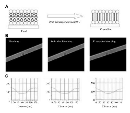
**Figure 5.** State change of diynePC as the temperature dropped to near 0°C. The diynePC changed from the fluid state to the crystalline state as the temperature dropped (A). In the FRAP experiment, a 40  $\mu$ m spot was bleached for 6 min, and then the fluorescence recovery was monitored after 5 min and 30 min (B and C).
